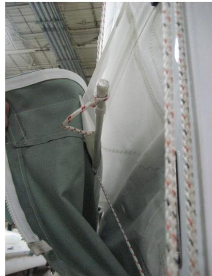
11. Tie off forward lazy jacks to lower pad eyes. Finish by seizing line ends with vinyl rigging tape. Note: Lazy jacks should not come in contact with rigging, shrouds, or any equipment.
