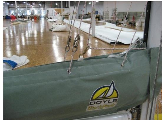
13. Aft reef line should be run up to reef point through reef slit on StackPack making sure that it runs outside of the Integral Membrane. (see photo above to right)
